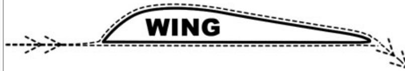
Look at the diagram above. Notice that the air traveling over the wing "hugs" the surface of the wing. Because of this, as the air leaves the wing it is traveling in a downward direction. Newton's third law states that for every action there is an equal and opposite reaction. So if the air is going down, the wing must go up.
