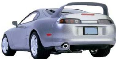
You may have noticed the race cars usually have spoilers on the back. Why do you think they are there? Draw a side view of a car (without a spoiler) and draw a dotted line showing how the air flows (like the side view of the wing above). You'll notice it is similar in shape to a plane's wing. Without the spoiler, is the downward travel of the air is "lifting" the back of the car making it lighter with less traction? How does the spoiler help with that?
